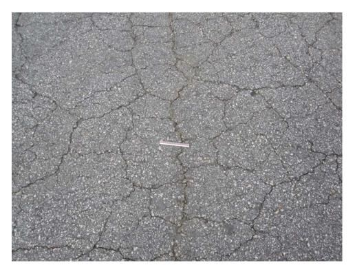
A03MR-10. Alligator Cracking (Sample Unit #14).
